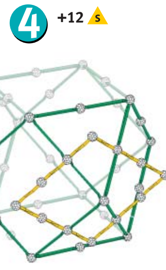
5 +60 s Continue to connect rhombuses around each vertex to complete the Rhombic Dodecahedron (5).
